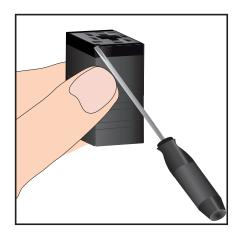
Figure 2 Connector Terminal Block Removal
